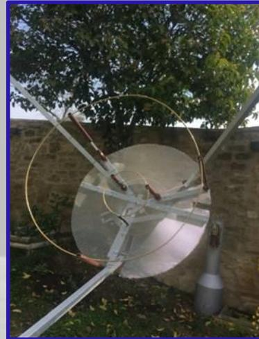
**Very easy access to the focus point that allows easy maintenance and fast feeder exchange.**
